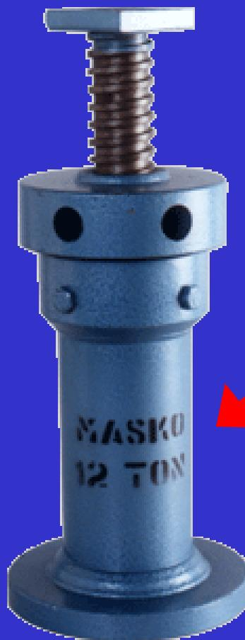
**The manufacturer's rated capacity must be marked on all jacks and must not be exceeded**
