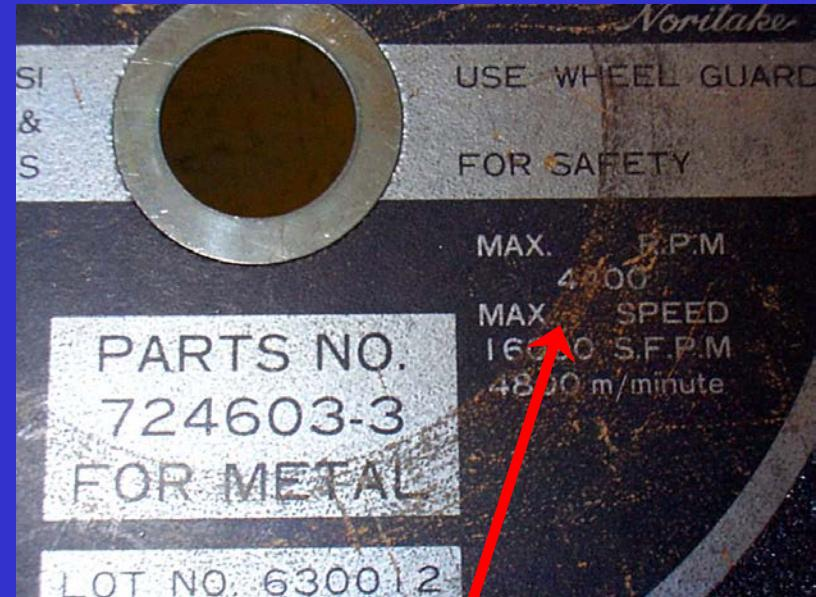
Ensure the spindle speed doesn't exceed the maximum speed marked on the wheel
